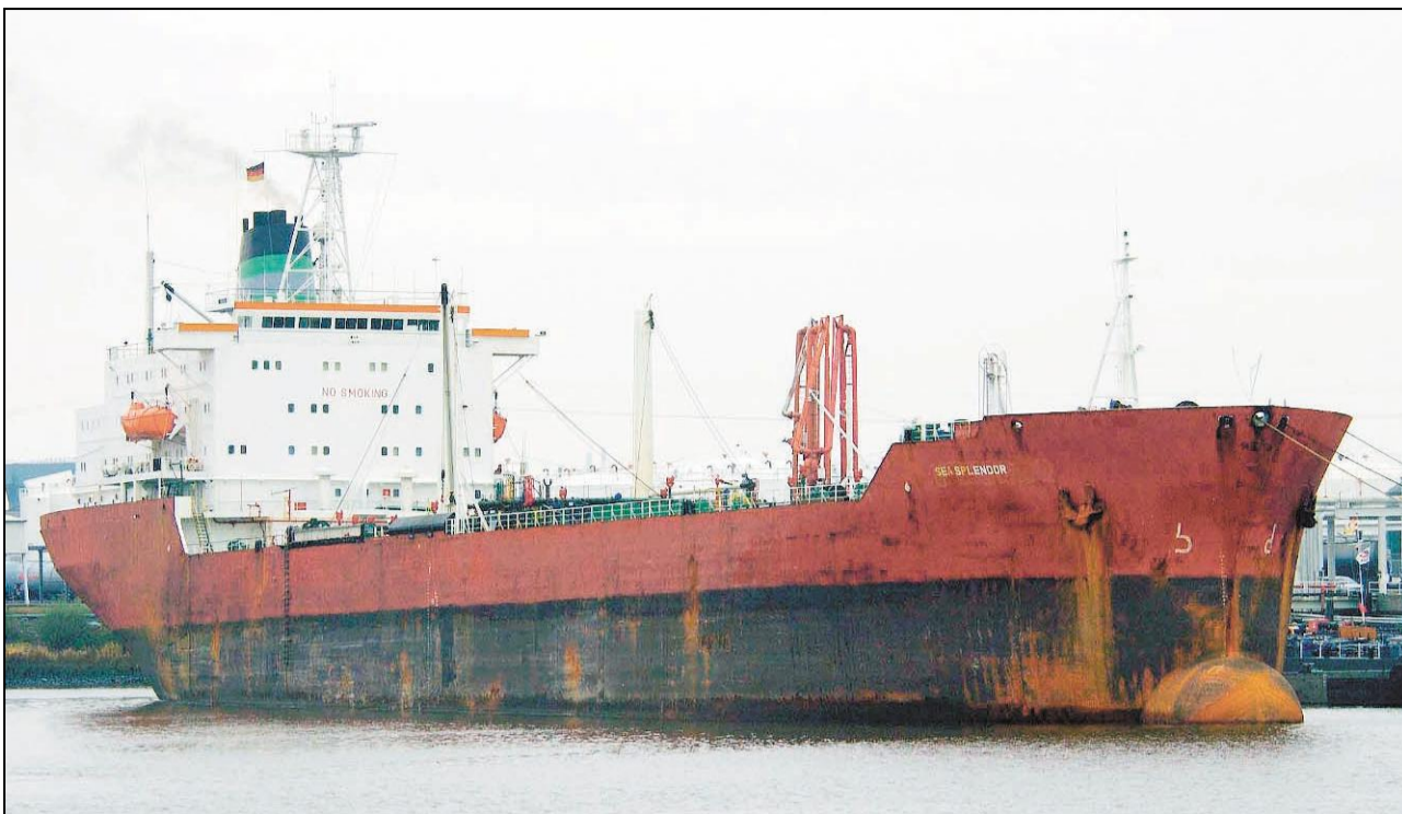
Dying breed: older single-hull vessels such as the 33,400 gt, 1977-built Sea Splendor face being phased out. Dietmar Hasenpusch
