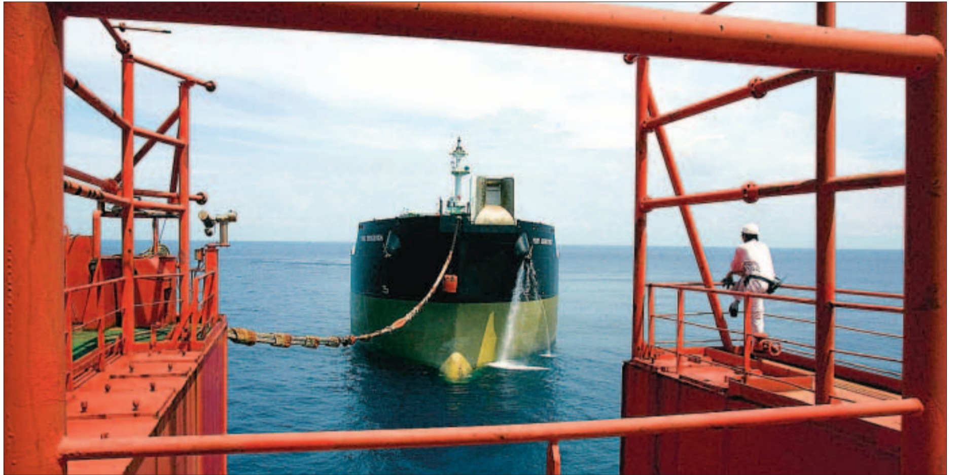
IN DEMAND: The 100,000-dwt tanker "Yuri Senkevich" (built 2005) sits connected to Bluewater's 103,000-dwt floating production, storage and offloading (FPSO) vessel "Munin" (built 1997) in the Lufeng oil field, South China Sea.
